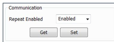
The node will now retransmit all received messages, depreciating the TTL by 1. If the received message has a TTL = 0, the message will not be retransmitted.
