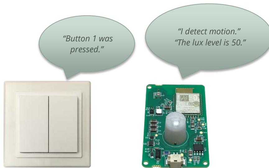
Each GalaXi node decides individually what to do in response to inputs from one or more sensors, switches, mobile devices, time clock, etc. These sensors and switches talk directly to the Xicato devices and do not pass through master controllers or gateways.
