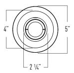
Ceiling Cut Out: 4 5/16" octagonal. Maximum Ceiling Thickness: 1 1/2"
