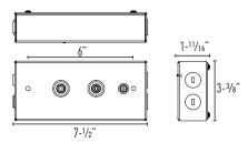
Remote driver box for eldoLED, Lutron  $^{\tiny{\textcircled{\scriptsize 0}}}$  & DMXR dimming options
