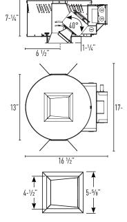
Ceiling Cut Out: 5-1/4" x 5-1/4" Maximum Ceiling Thickness: 1-1/4" Minimum Ceiling Thickness: 1/2"
