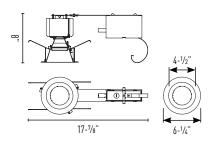
Ceiling Cut Out: 5-1/4" Maximum Ceiling Thickness: 1-1/2" Minimum Ceiling Thickness: 1/2"
