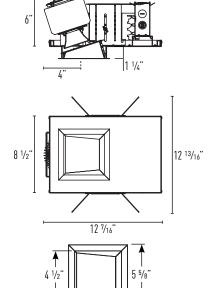
Ceiling Cut Out: 5 1/4" x 5 1/4" Maximum Ceiling Thickness: 1 1/4" Minimum Ceiling Thickness: 1/2"
