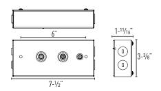
Remote driver box for eldoLED, Lutron® & DMXR dimming options
